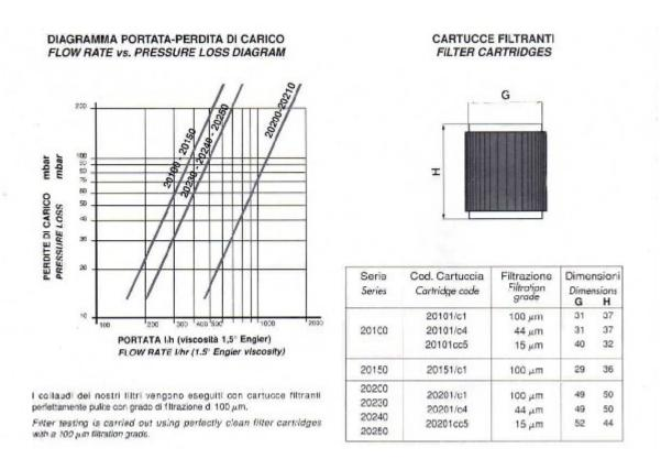
Filter testing is carried out using perfectly clean filter cartridges with a 100 µm filtration grade.
